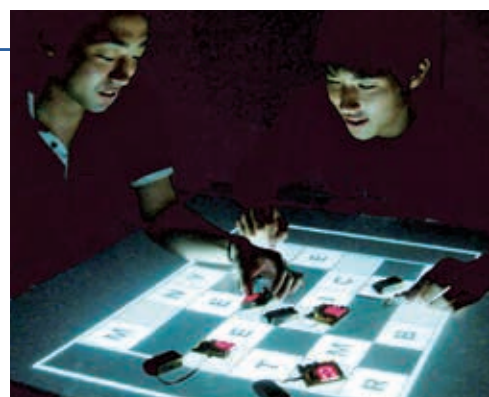
"EmiTable", a table-type display that reveals hidden light signals as visible pixel units.
