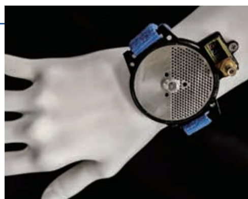
Electret device generating electricity from arm movement
